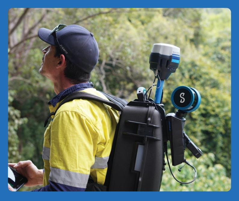
Emesent's Backpack RTK automates georeferencing and drift-correction for backpack-based scans to deliver fast, accurate and precise scans — without the need to lay out and georeference ground control points.
